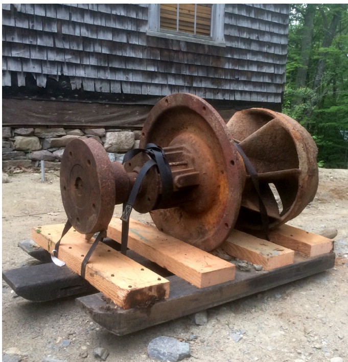
Wetmore turbine before repair, June 2018.
