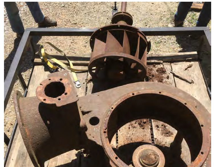
Display turbine donated by Kmiec family shows runner with shaft, case with lignum vitae bearing in center.
